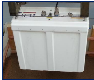
Fig. 3 Air-coupled 2 GHz horn antenna
