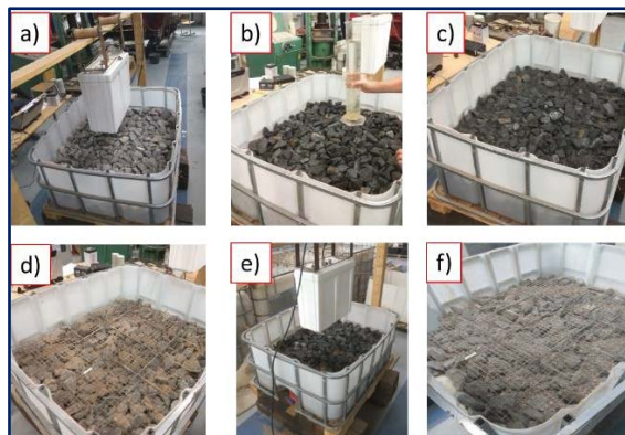
Fig. 4 Test configurations for a) clean dry ballast, b) gradual addition of water to clean ballast via measuring cylinder, c) fully saturated ballast, d) dry ballast fouled with sand, e) wet ballast polluted with sand f) dry ballast fouled with fine gravel
