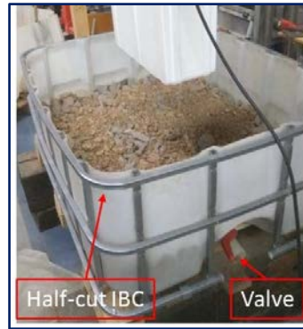
Fig. 2 Half-cut IBC with the drain valve
