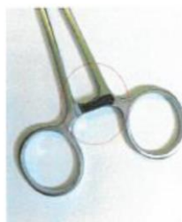
Fig. 1 Putting RFID chip into the resin mixture directly on the surface of the tool [18]
