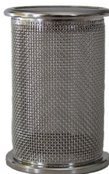
Figure 7: Rotating basket for dissolution tests [26]
