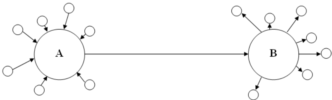
Obrázek 5: Princip metody Hub and Spoke
