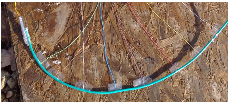
Figure 4. The detonating cord with 8 glass fibres inserted into the PETN core as used in Experiment 1
