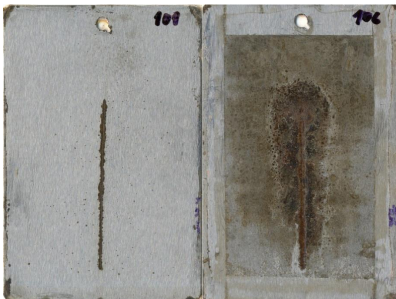
Figure 10 Corrosion in the cut: (left) Mg 0.2 Zn 0.8 Fe 2 O 4 /Zn pigment with lamellar particles at PVC 10%; (right) Mg 0.2 Zn 0.8 Fe 2 O 4 pigment with isometric particles at PVC 10%
