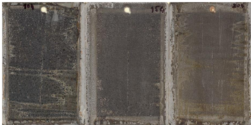
Figure 9 Example of metal surface corrosion beneath a paint film with the isometric \text{ZnFe}_2\text{O}_4 ferrite at PVC A)10%, B)15% and C)20% after 2100 hours exposition
