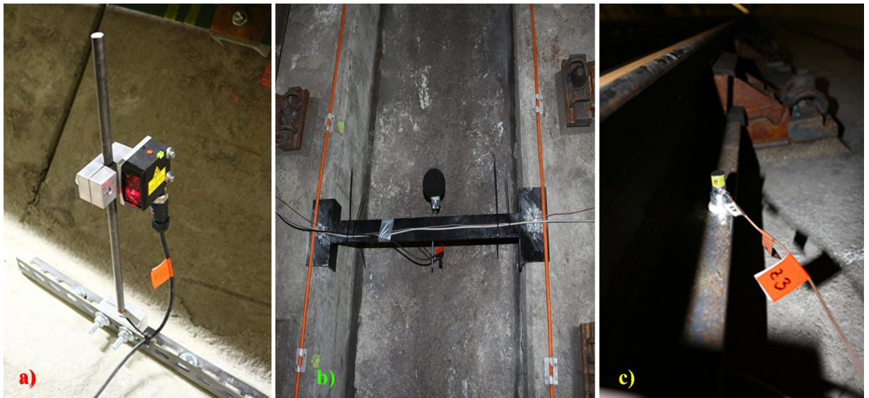
Figure 2: Balluff BOS016U optical gate (a), Kistler 8702B100 acoustic sensor (b), Brüel & Kjær 4188 vibration sensor (c) (author: Vágner J.)
