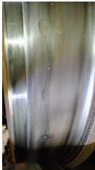
Figure 27: Wheel flat which is present on the seventh wheelset on train set ID-108
