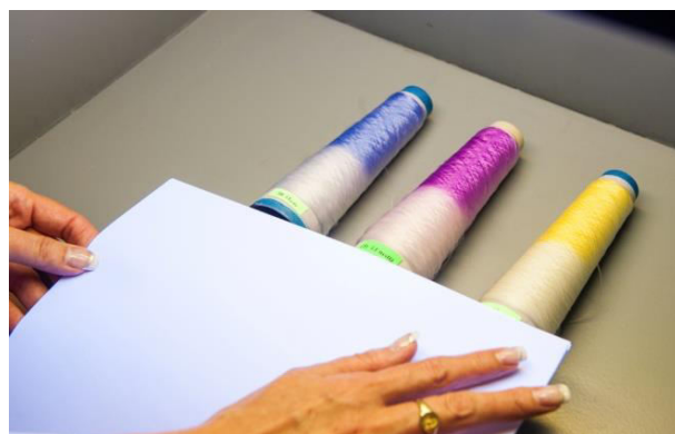
Figure 2 Samples of photochromic polypropylene multifilament
