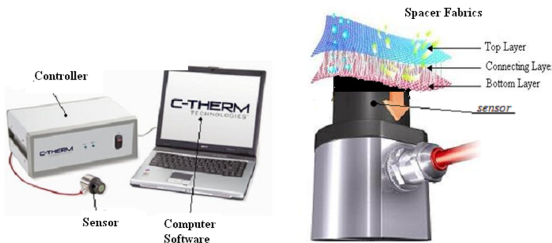
Figure 1 Thermal conductivity (Tci) analyzer (C-Therm)
