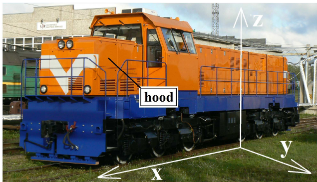
Fig. 1 Coordinate system according to EN 12663-1
