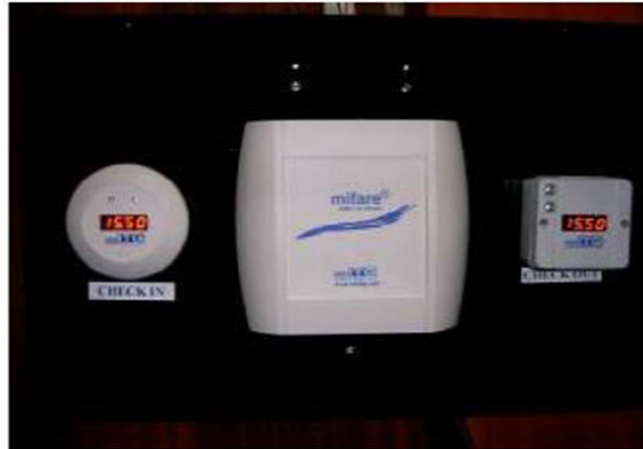
Fig. 6. Terminal device reader (CHECK IN or CHECK OUT)
