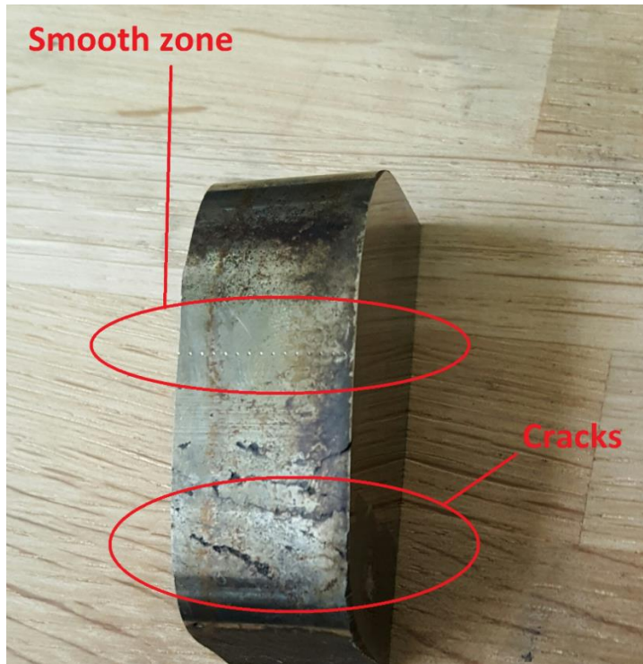
Figure 50 Sample was tested 2 points from different zones: smooth zone crack zone
