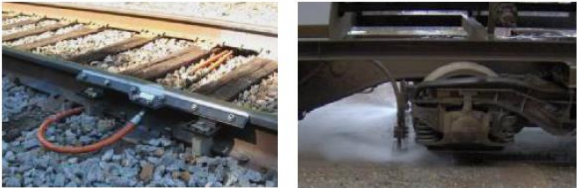
Figure 2 Water jetting to prevent slide [10].
