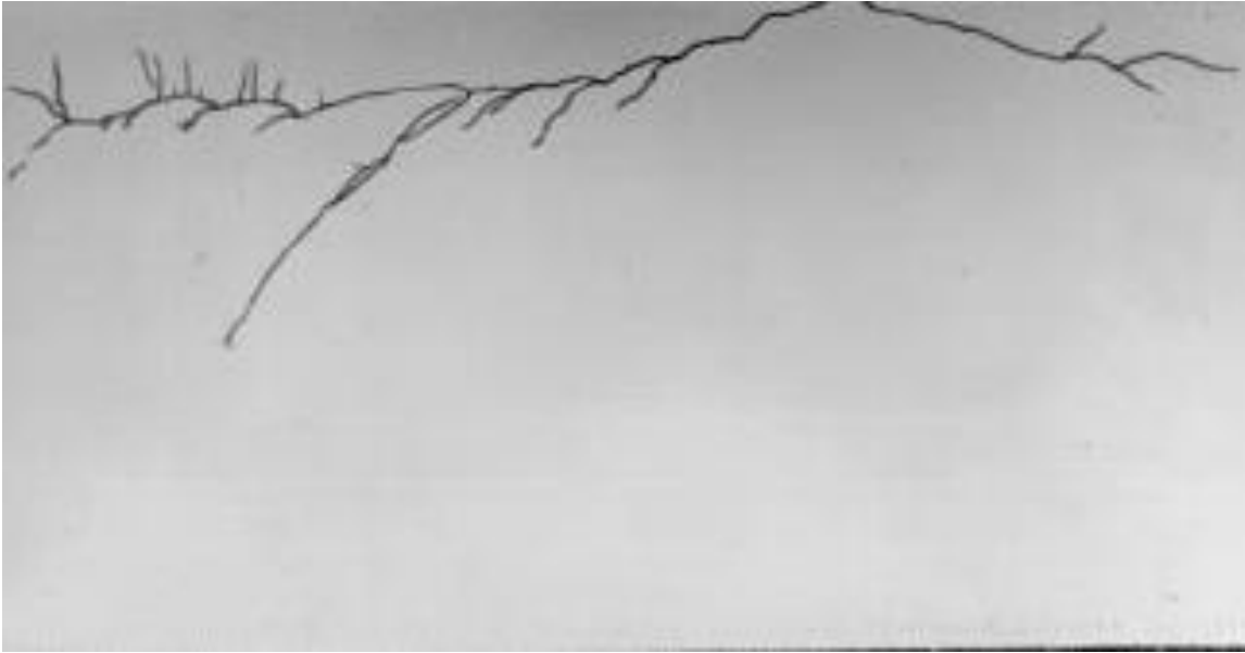
Figure 15 Squats results sub- surface cracks which propagates in travel direction and opposite direction [CD s 67]
