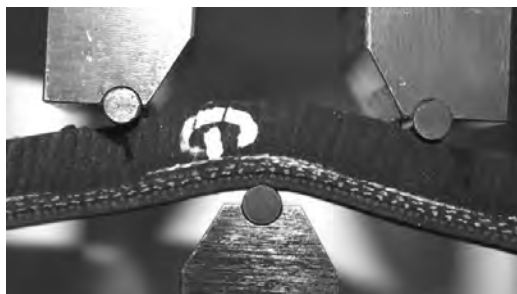
Fig. 2 Specimens in radial direction with tread after bending loading
