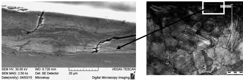
Figure 2 Creation of the well and microcracks.
