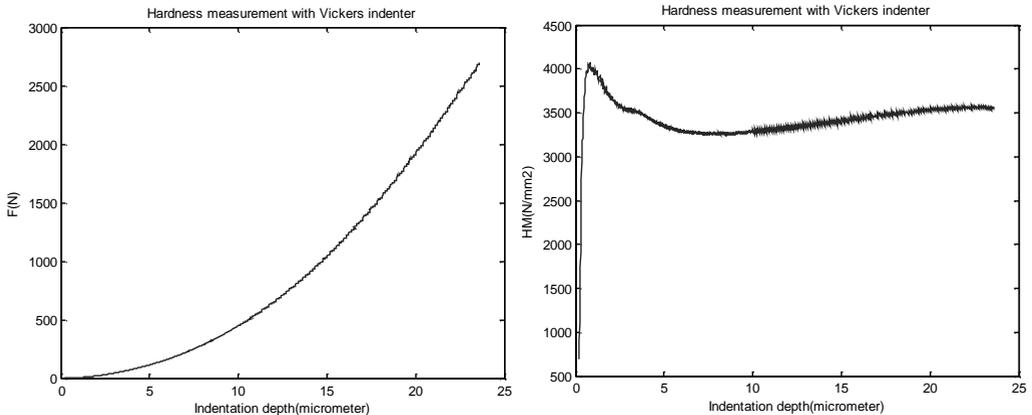
Figure 5 Physical behavior of Hadfield steel under Vickers indentation.
