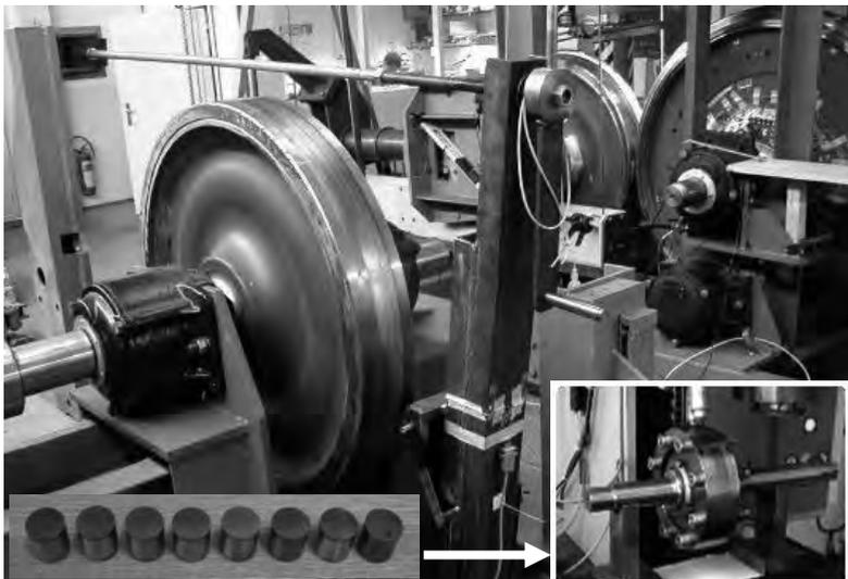
Figure 1 Rolling-contact fatigue testing equipment, detail on holder for set of tested samples
