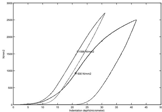
Figure 4 Finding Comparative yield stress CYS [ $\text{N/mm}^2$ ] by using cylindrical indenter (red line explosive hardening, blue line without exp. hardening)
