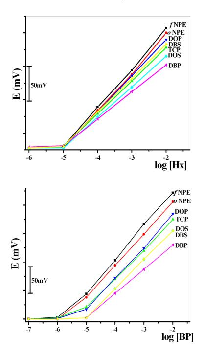
Fig. 3: Effect of the plasticizer on the performance of Hx and BP sensors.
