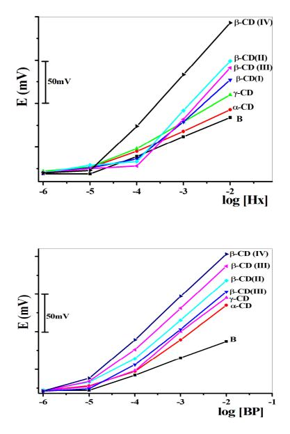
Fig. 1: Effect of the sensing ionophore on the sensor performances.
