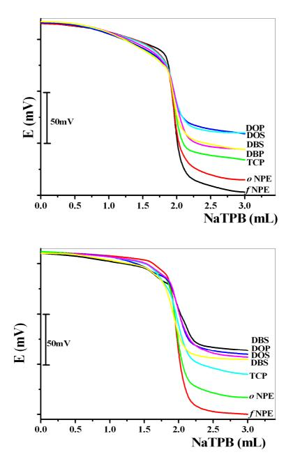
**Fig. 4**: Effect of the membrane plasticizer on potentiometric titration of 2 mL  $10^{-2}$  mol·L<sup>-1</sup> Hx and Bp solutions with  $10^{-2}$  mol·L<sup>-1</sup> NaTPB.
