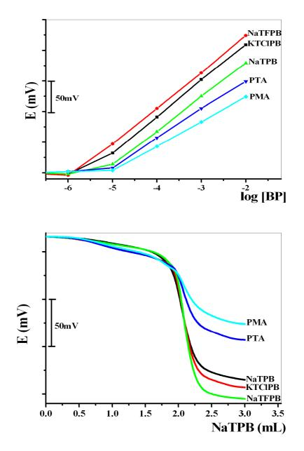
Fig. 2: Effect of ionic sites type on BP sensor performance.
