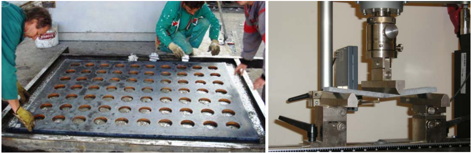
Fig. 6 Application of studied composite for the heating core of the structural member (left); configuration of the three-point bending test (right)
