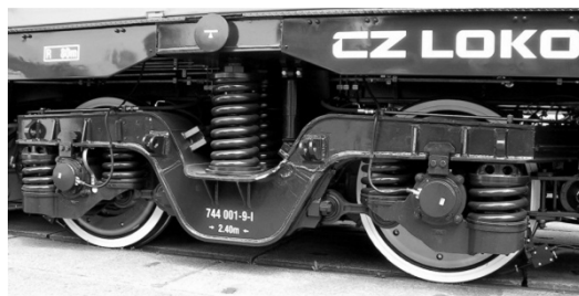
Obr. 2 Podvozek lokomotivy řady 744.0 Fig. 2 Bogie of the locomotive Class 744.0
