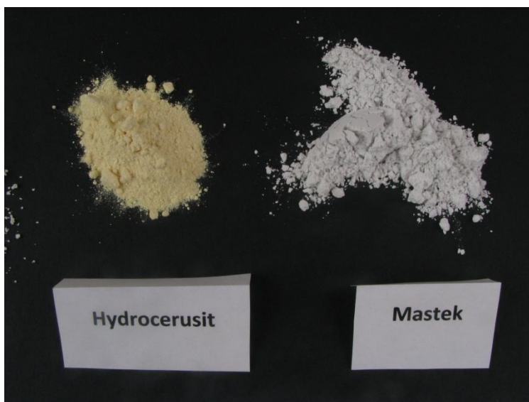
Obr. 194 Hydrocerusit a mastek
