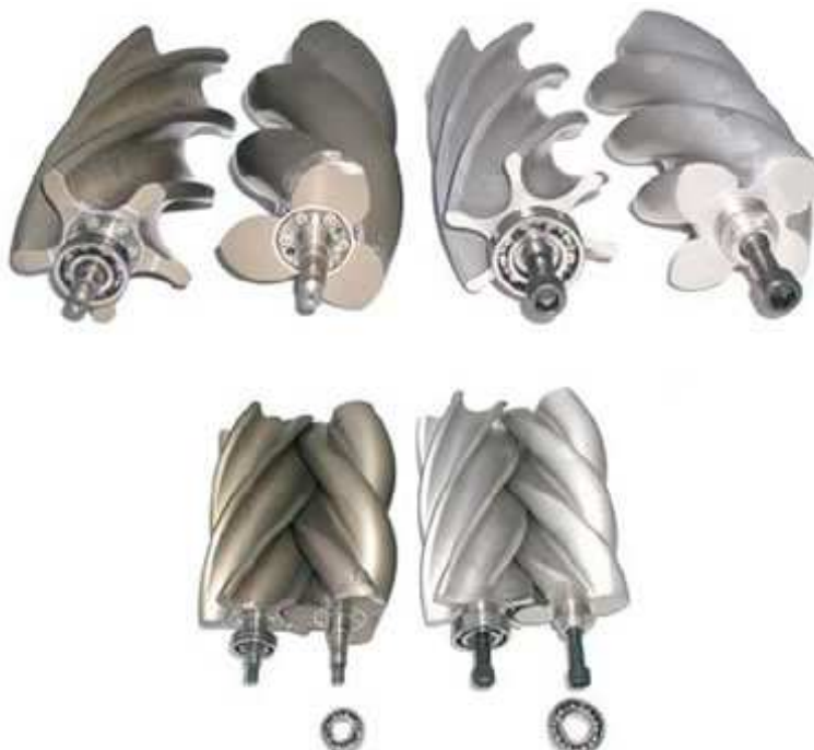
Obr. 20: Rotory Lysholmova dmyhadla [7]
