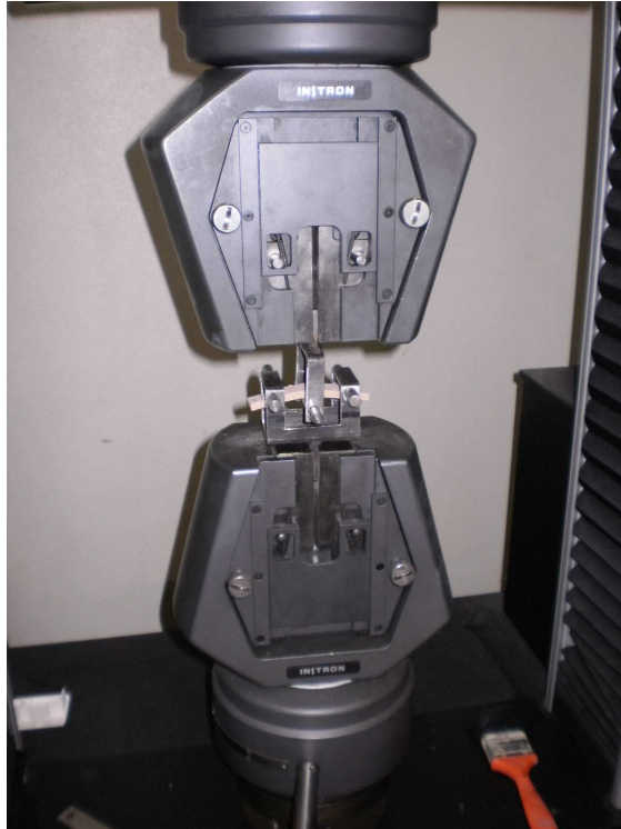
Fig. 3 Bending device (3-point method) of the testing machine
