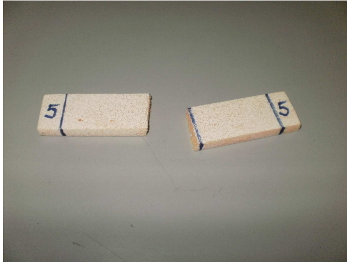
Fig. 5 Failure of individual specimens in the middle of the panel
