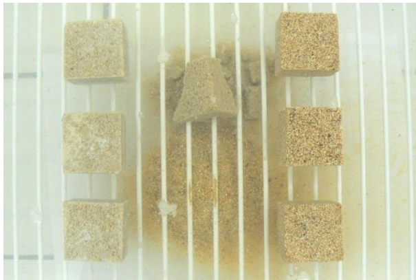
Figure 39. Specimens during 1 st cycle of freeze-thaw test. Not consolidated substrates (in the middle) disintegrated immediately after immersion into the water container.
