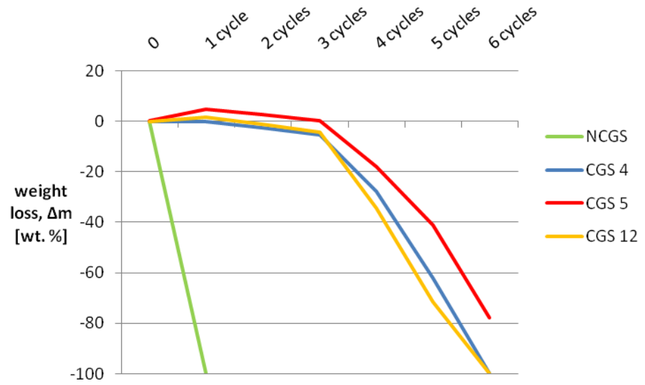
Figure 45. The weight change of not consolidated (NCGS) and consolidated (CGS) gypsum substrates during the salt crystallization test by capillary action.
