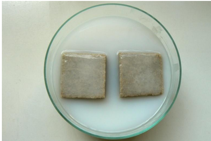
Figure 9. The gypsum substrates during consolidation by immersion in Sol \text{CaSO}_4\text{-Ca(OH)}_2 .
