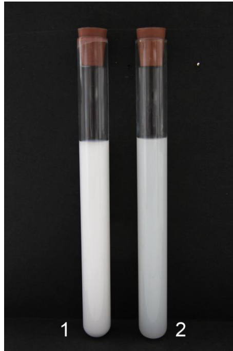
Figure 11. Nanosuspension CaLoSil® E25 (1) and Sol CaSO 4 -Ca(OH) 2 (2)
