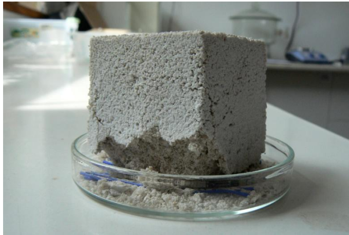
Figure 54. The substrate (CGS) after one week of the outside exposition.
