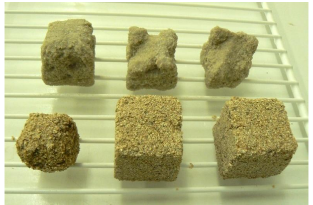
Figure 40. Specimens after 5 th cycle of freeze-thaw test.
