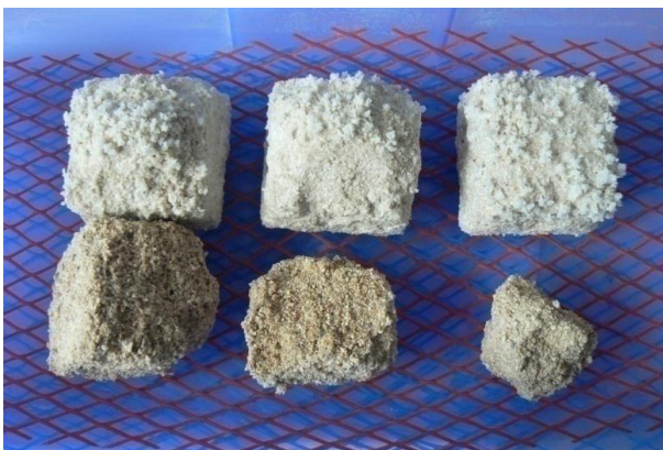
Figure 48. Salt crystallization test by immersion. The substrates after 2 st cycle.
