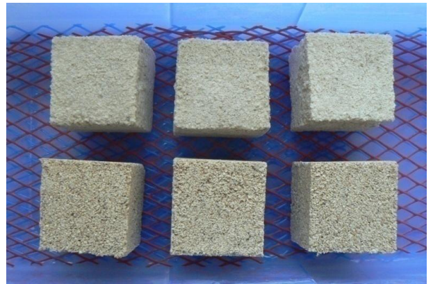
Figure 47. Salt crystallization test by immersion. The substrates after 1 st cycle.
