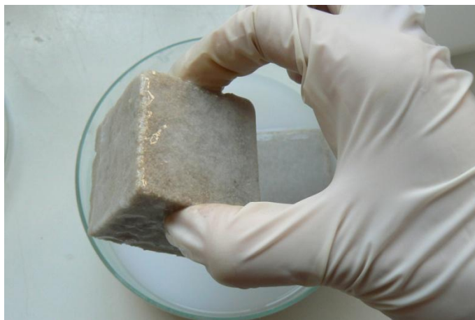
Figure 10. The gypsum substrate after removing from the consolidation bath.
