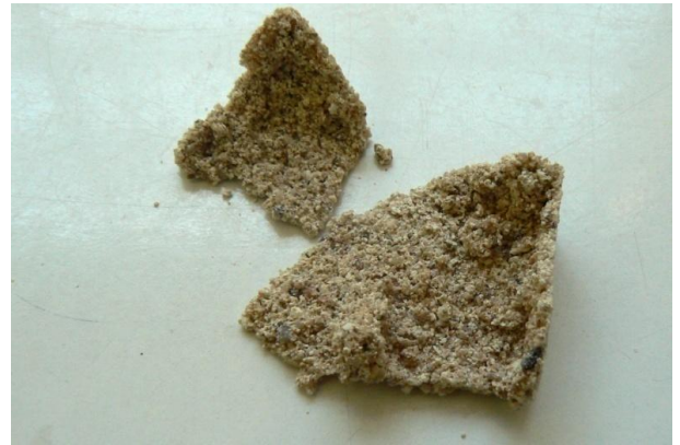
Figure 51. The crust created on the lime specimen. Salt crystallization test by capillary action. The substrate after 3 th cycle.
