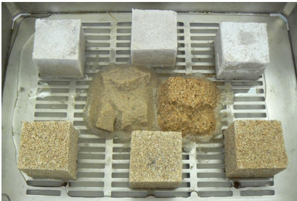
Figure 46. Specimens during 1 st by capillary action. Not consolidated substrates (in the middle) disintegrated immediately in contact with salt solution.
