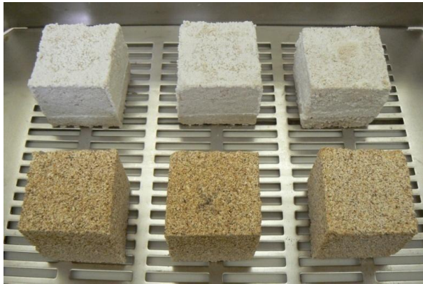
Figure 50. Salt crystallization test by capillary action. The substrates after 1 st cycle. The white colour of gypsum specimens is caused due to the presence of small crystals layer on the surface.
