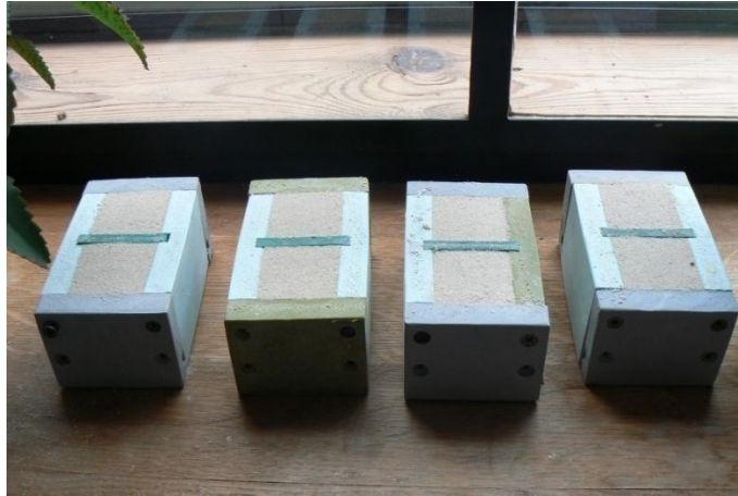
Figure 6. Prepared samples were drying in the moulds.
