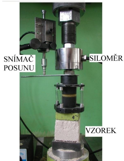
Figure 17. The compression strength testing device. The picture was made by ITAM AS CR v.v. i Prague.
