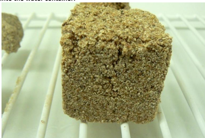
Figure 41. Cracking and rupturing of CLS specimen after 6 th cycle of freeze-thaw test.
