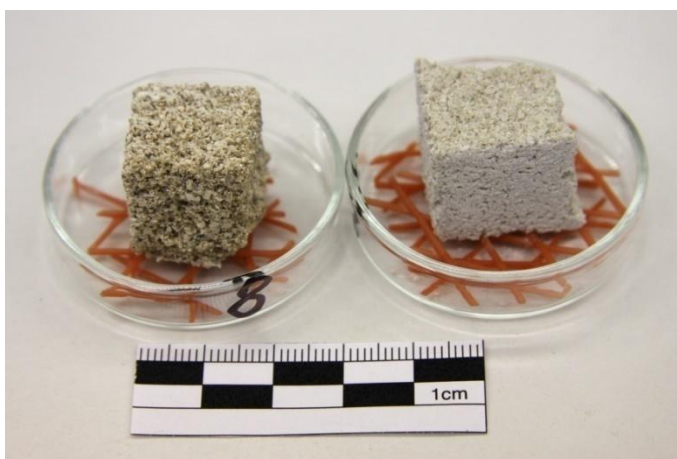
Figure 19. Specimens (cubes 2 \times 2 \times 2 \text{ cm}^3 ) for water vapour adsorption test.
