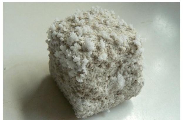
Figure 49. The formation of salt crystals on the top of the gypsum specimen. The substrate after 2 st cycle of immersion.
