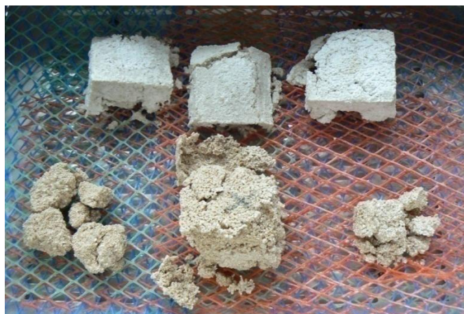
Figure 52. Salt crystallization test by capillary action. The substrates after 4 th cycle.
