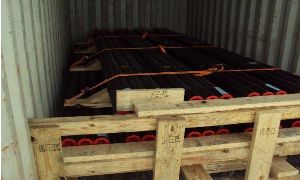
Figure 16: Blocking braces Source: (12)
