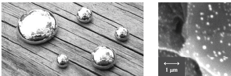
Fig. 1: Due to a high surface tension, liquid mercury readily forms compact droplets; regardless if the resultant aggregates are large drops at a wooden desk (left) or tiny droplets in the nanometer scale as the film deposited onto a carbon paste surface (right) [Illustrative photos from authors' archives]
