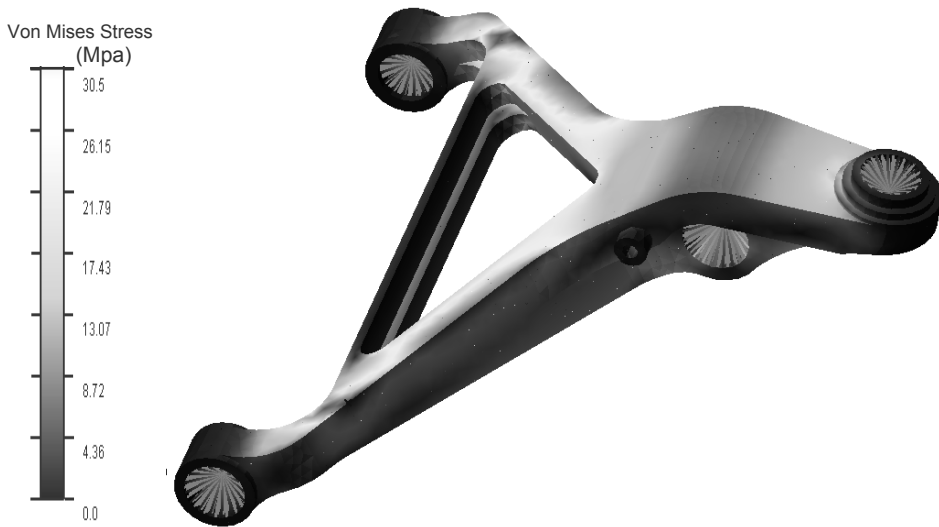
Fig.10 Stress distribution in lower arm
