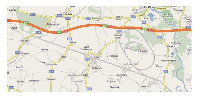
The Poříčany - Kolìn pilot section, 22 km long, represents a ERTMS/ETCS Level 2 system application, according to the UNISIG SRS version 2.3.0 (Subset-108 version 1.0.0).
