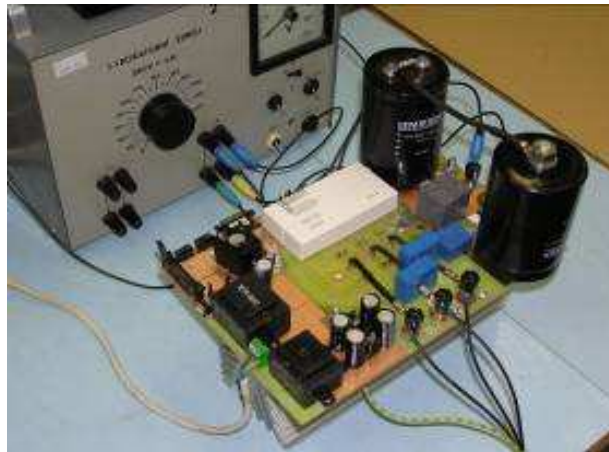
Fig. 2 Experimental IGBT invertor for high speed drive
