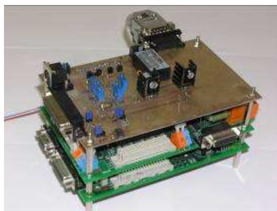
Fig. 3 DSP controller of high speed drive with TMS320F2812 and with additional unit for PMSM rotor angel position evaluation
