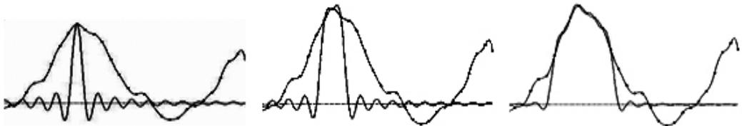
**Fig. 2** The original signal and its approximation by one; three and eight elements of the Shannon basis
