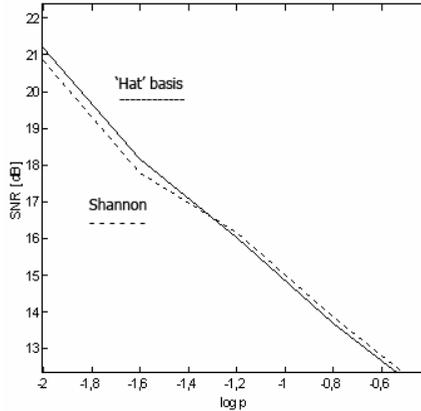
**Fig. 7** Results of the simulation for the SNR in case of 'hat' decomposition.
