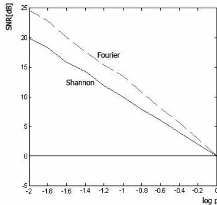
**Fig. 6** Results of the simulation for the SNR in case of Shannon and Fourier decomposition.
