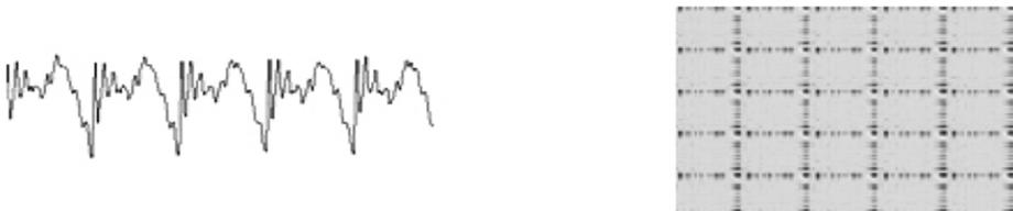
**Fig. 3** The real sound of vowel 'E' running 20 ms. The mean as a function of time and correlation as a two dimensional function of time variables.
