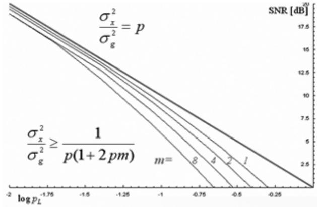
**Fig. 5** Limitation for SNR in case of basis  $B_1, B_2, B_4, B_8$
