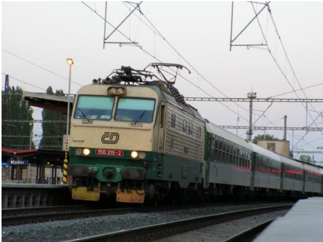
Obr. 1 Lokomotiva 150 215-2 (ŠKODA 65 E 1)
