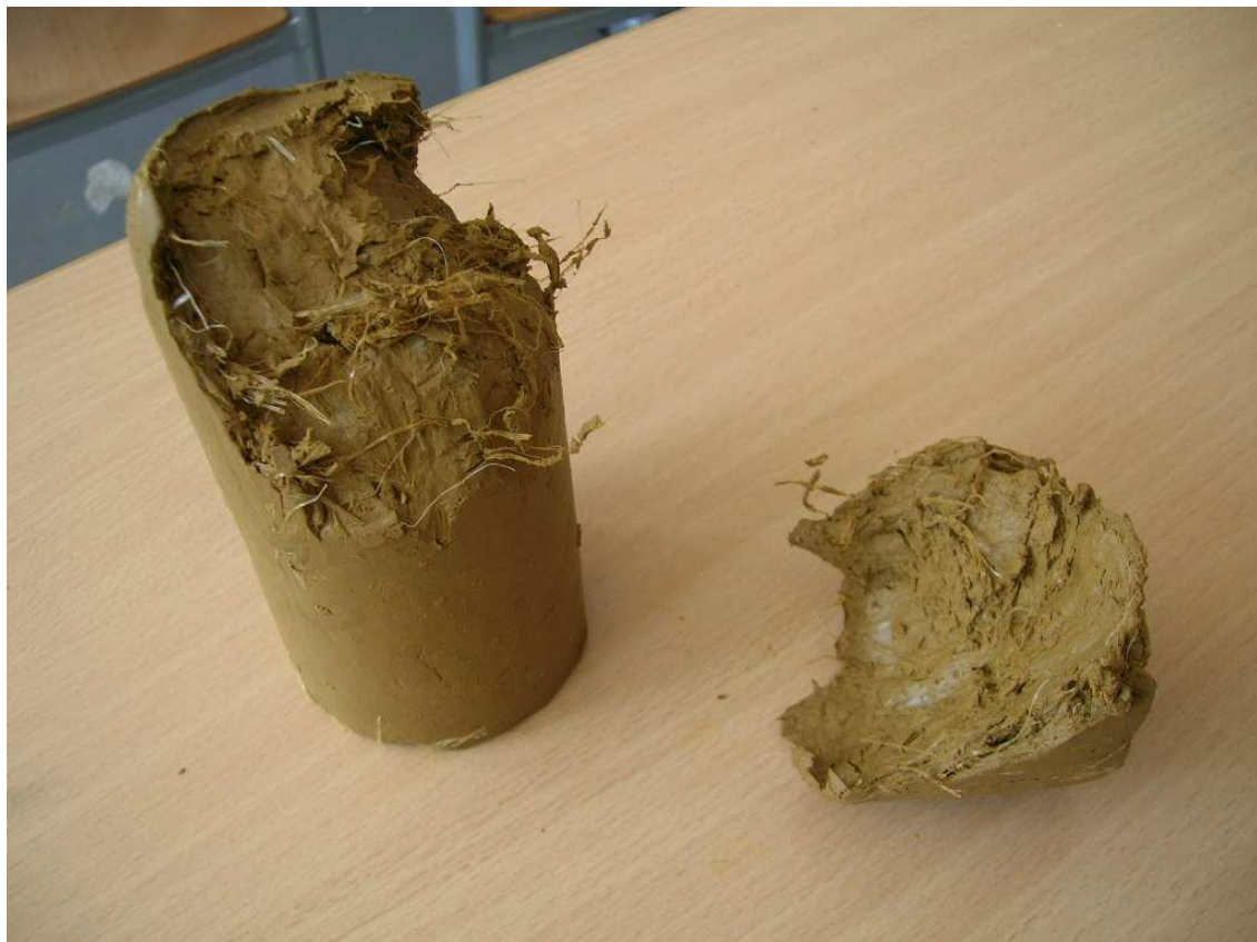
Figure 6-26. Shear breaking plane, reinforced specimen [0]
