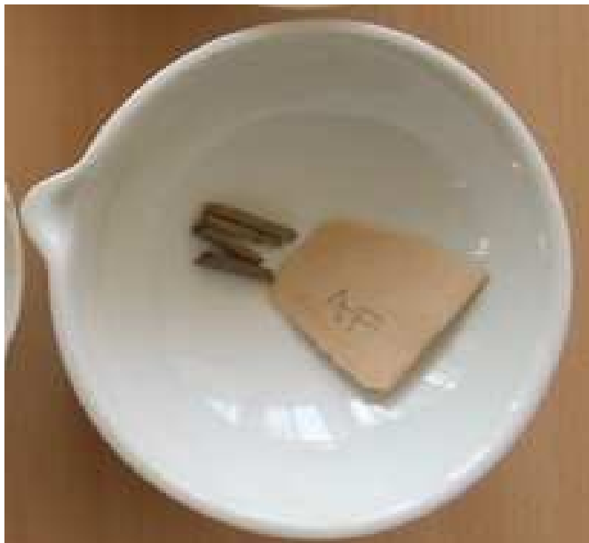
Figure 4-4. 3 mm diameter threads, test of plasticity on the thesis' sample [0]
