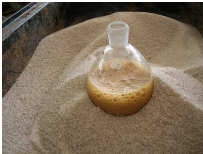
Figure 4-7. Pycnometer with boiling suspension in a sand bath [0]
