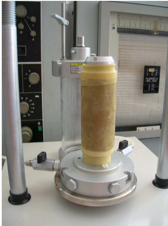
Figure 4-13. Specimen prepared for triaxial test [0]
