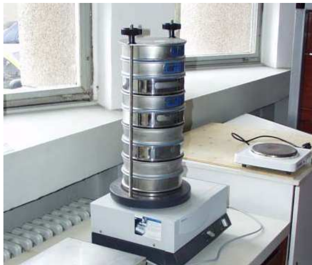
Figure 4-2. Apparatus and stack of sieves for grain size distribution test [0]
