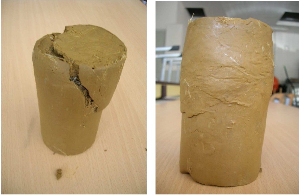
Figure 6-25. Reinforced specimens after triaxial test (1) unconfined (2) confined compression [0]
