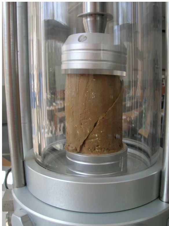
Figure 4-12. Shear breaking plane, unconfined compression test of the thesis' sample [0]
