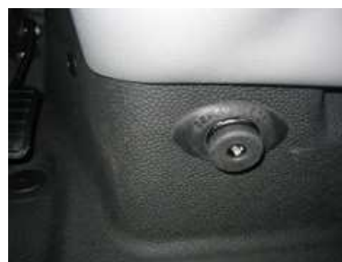
Obr. 16 Defend Lock – Push Lock [3]
