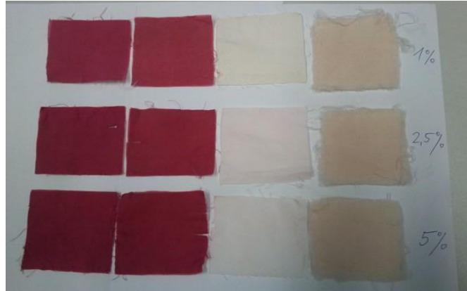
Figure 41. Dyed material: 100 % cotton with FA-BQPER 2.
