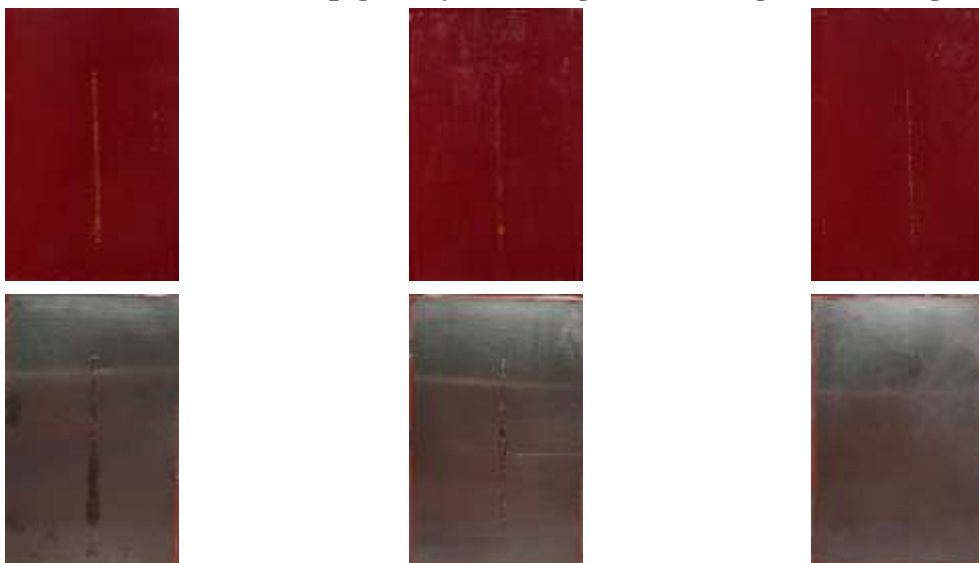
OP s \text{ZnO} , \text{Fe}_2\text{O}_3 a pigmenty \text{C}_{12}\text{H}_6\text{MgO}_4 , \text{C}_{14}\text{H}_4\text{Mg}_2\text{O}_4 a \text{Ca-Mg-HPO}_4
