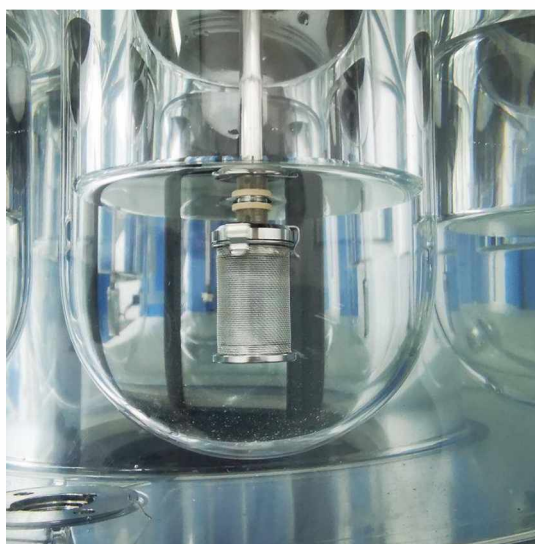
Figure 21: Rotating basket method. [92]
