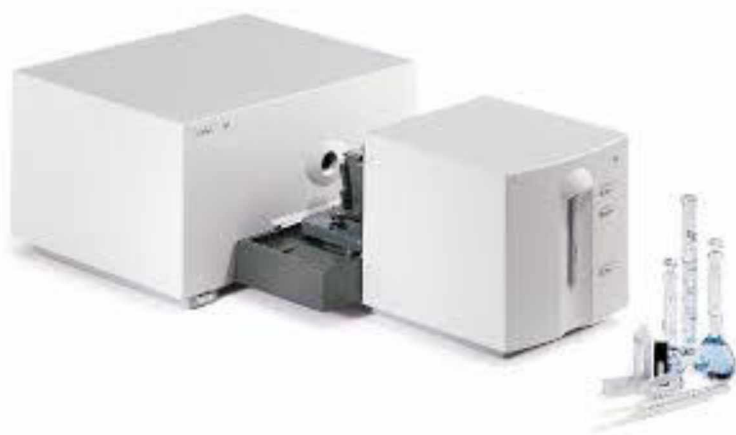
Figure 25: UV/VIS spectrophotometer - Agilent 8453. [95]
