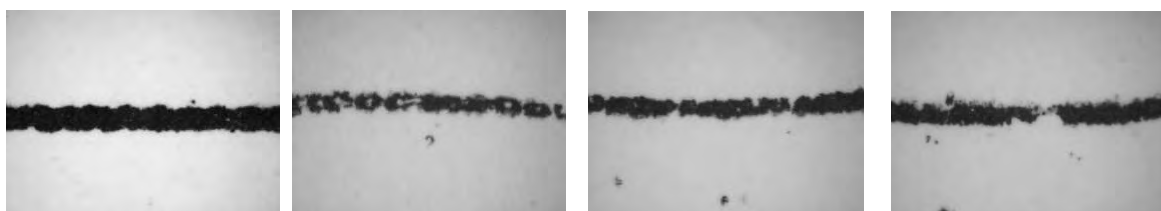
a) line 1 single printed b) line 1 double printed c) line 1 triple printed d) line 2 single printed
