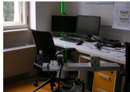
Fig. 1: The rotary 3D range scanning system
