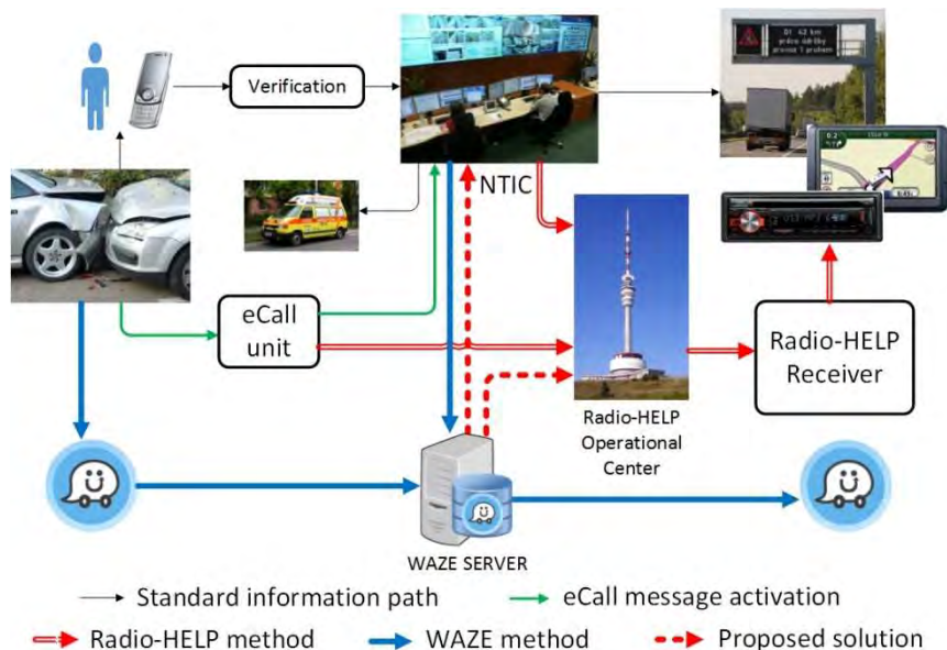
Fig. 1: Transmission and acquisition of information in the event of an accident with the use of the eCall, Radio HELP and WAZE)
