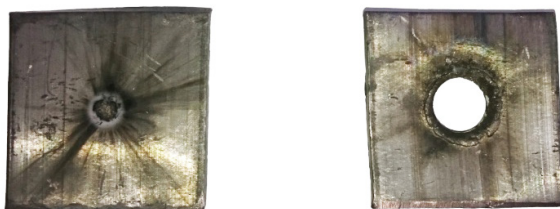
Figure 6. Witness lead plate test: 200 mg AgTNADAzT (left), 10 mg dextrinated lead azide (right)
