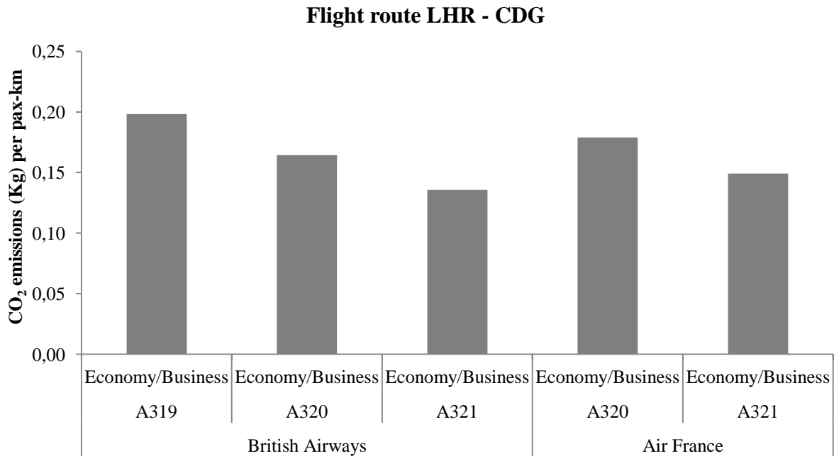
Figure 33 Comparison of carbon dioxide emissions per passenger-kilometre between aircraft used by British Airways and Air France in daily flights between LHR and CDG.
