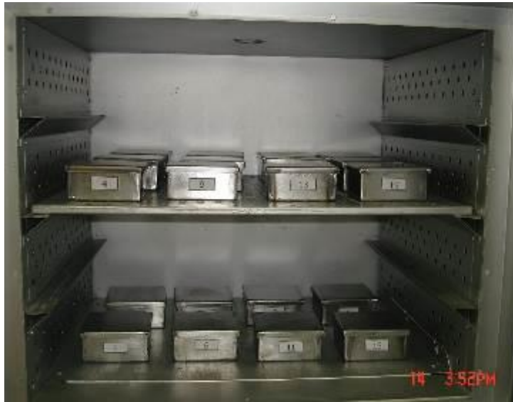
Figure 29 - Oven at 40 °C – during 30 days
