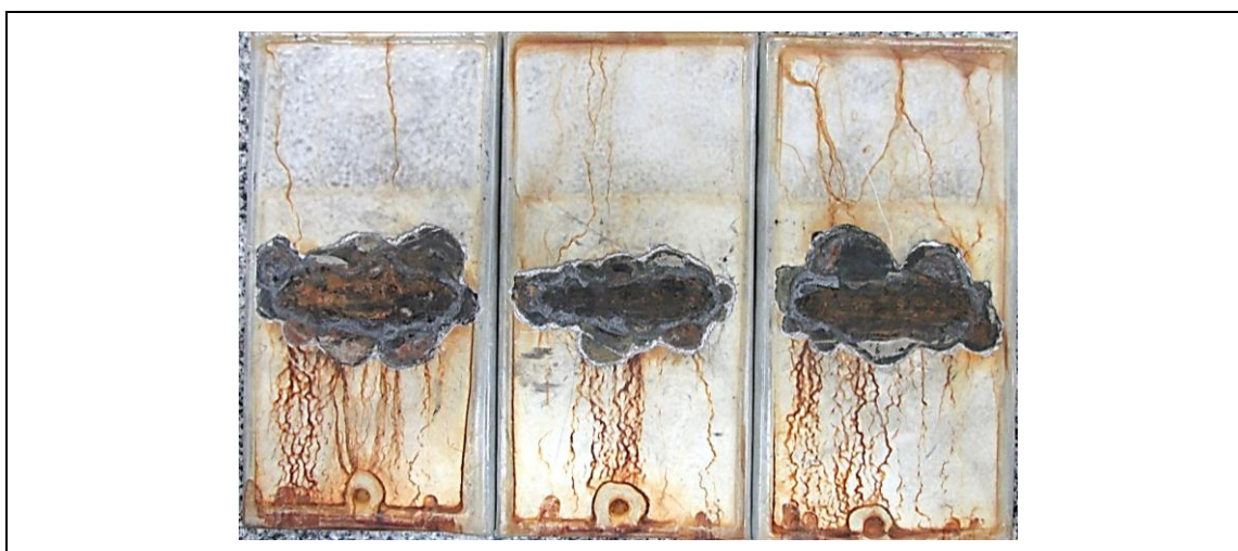
Figure 51d – Samples 07, 08 and 09 (SPH1712 dry) – after 20 cycles Cyclic Corrosion Test
