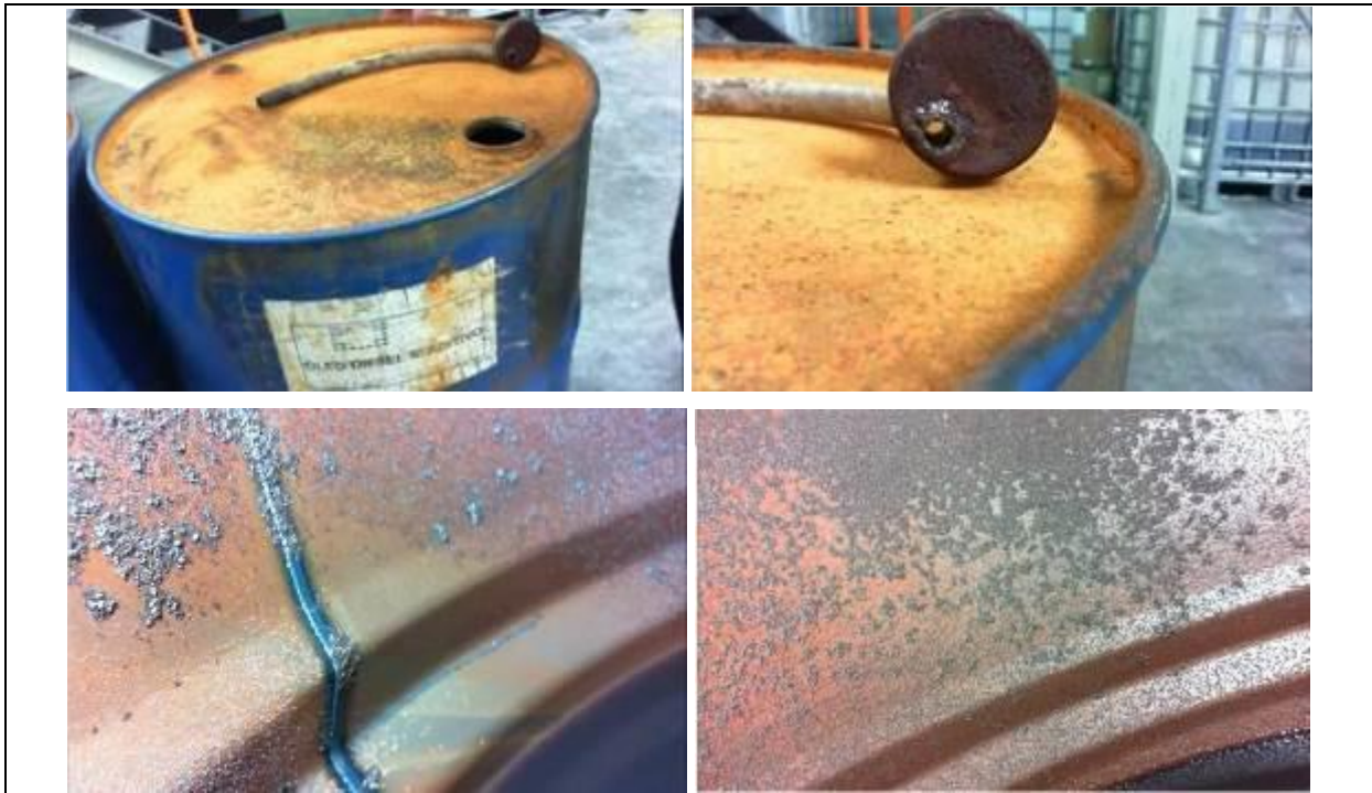
Figure 36 – 200L Drum with diesel and without corrosion inhibitor
