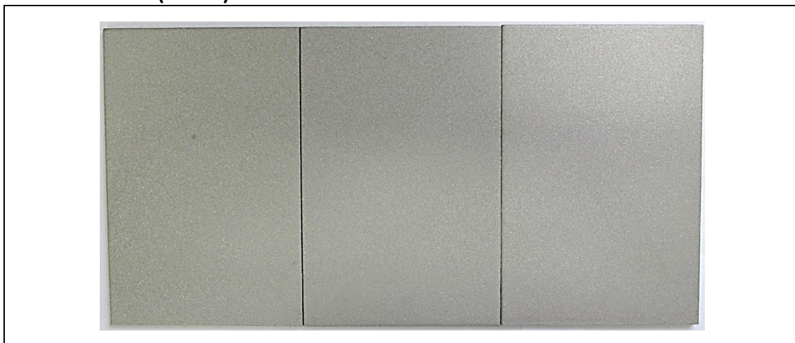
Figure 49a – Condition Jet – 1, 2 and 3 – flash rust test – initial (time 0)
