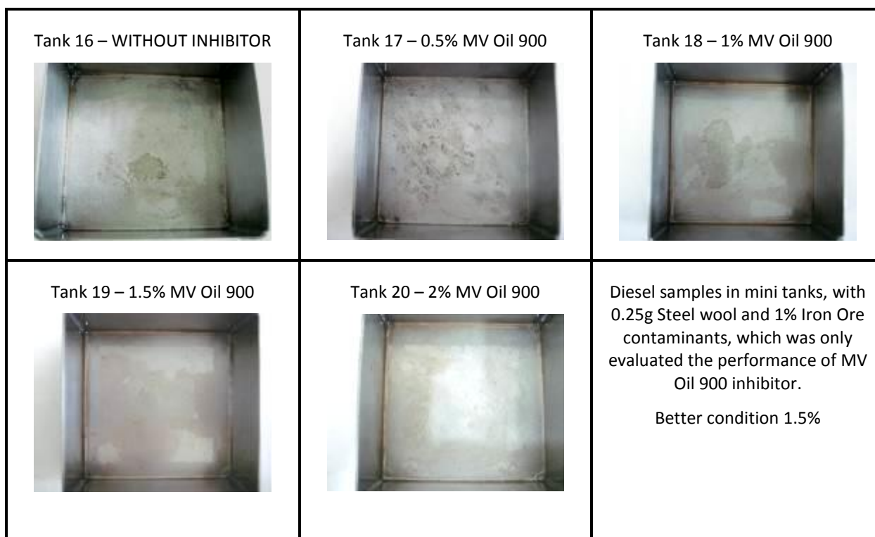
Figure 33 – Results sequence for mini tanks with diesel and with Iron ore and with 0.25 g of steel wool contaminant and MV Oil 900
