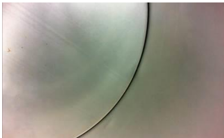
Figure 41 – Top of the Drum with diesel and with 0.5% of V-active VCI1061 corrosion inhibitor – clean
