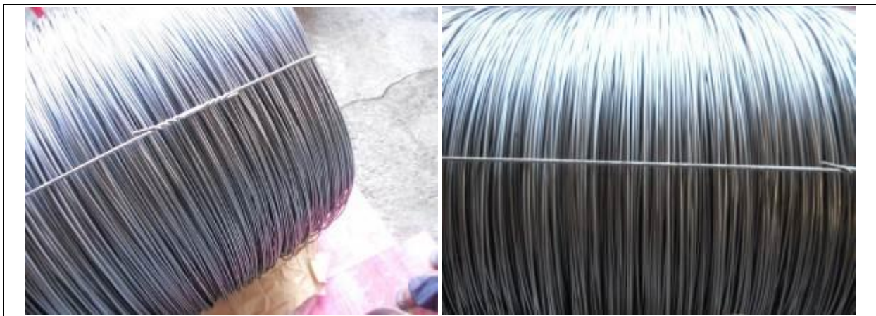
Figure 70 – Wire Steel Coil after 43 days – side condition
