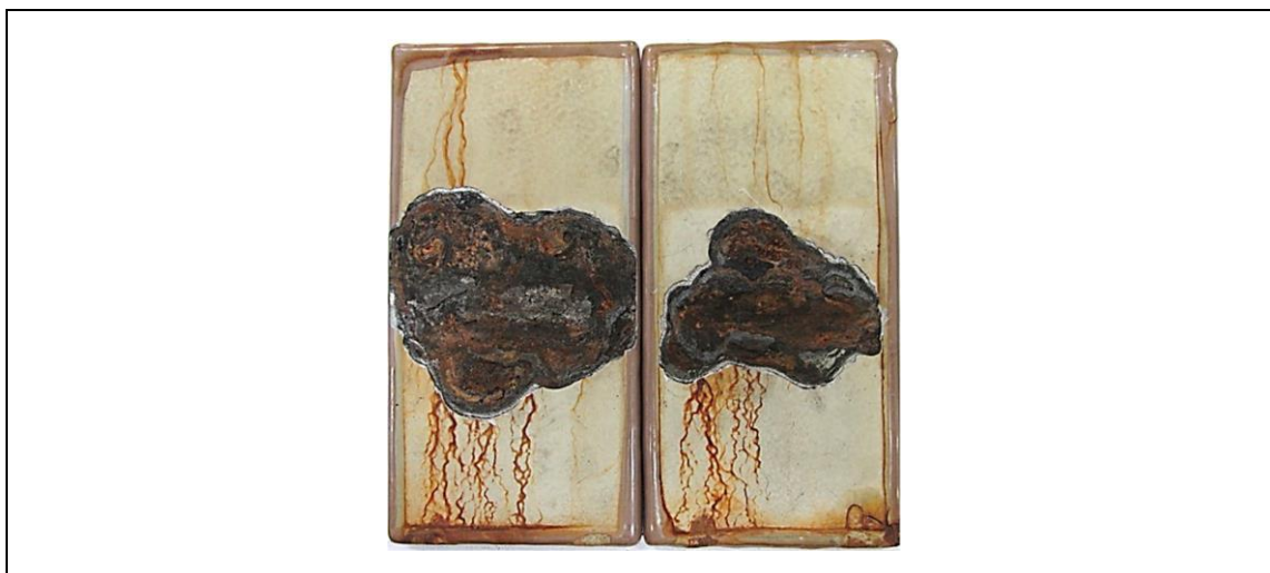
Figure 51a – Samples 69 and 70 (Jet condition without inhibitor) – after 20 cycles Cyclic Corrosion Test
