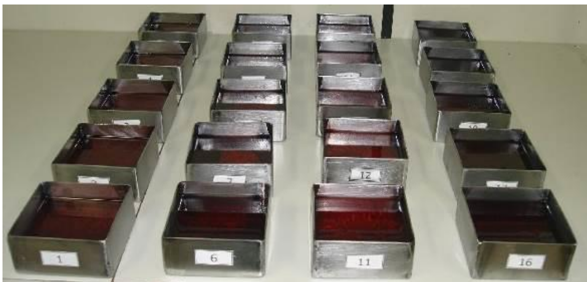
Figure 28 – Mini tanks, with 250mL of diesel fuel, added with MVOil900, water, Iron ore and steel wool
