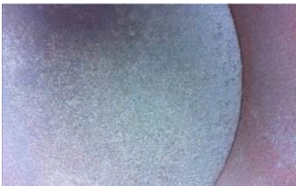
Figure 38 – 200L Drum with diesel and without corrosion inhibitor: intense corrosion at the upper (top).
