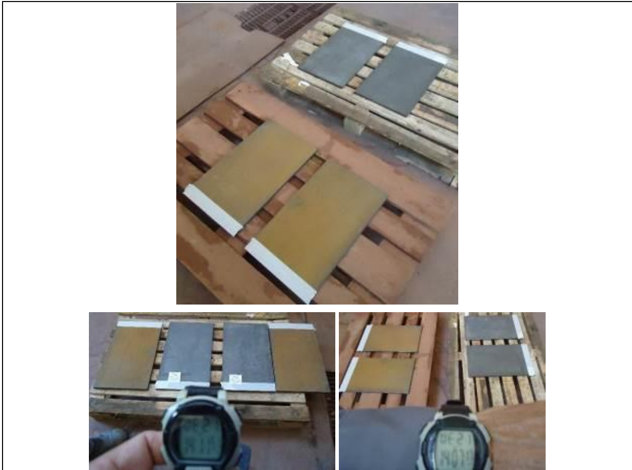
Figure 46 – Steel plates – after hydrojetting – 5 hs later – without corrosion inhibitor presence of flash rust
