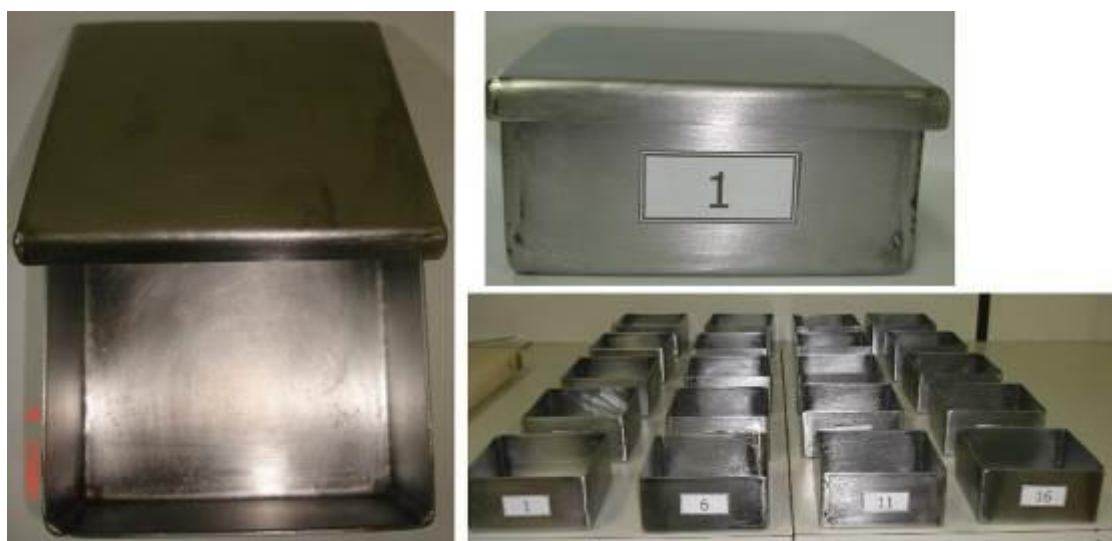
Figure 26 – Mini tanks made with steel 1020
