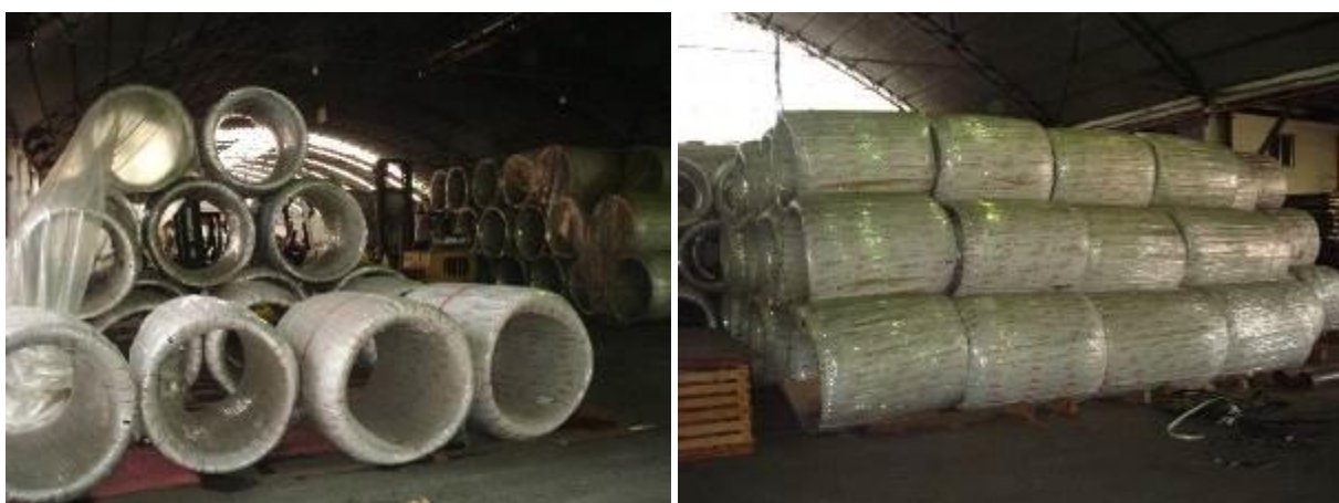
Figure 55 – Storage condition of the wire steel coils before loading of the containers
