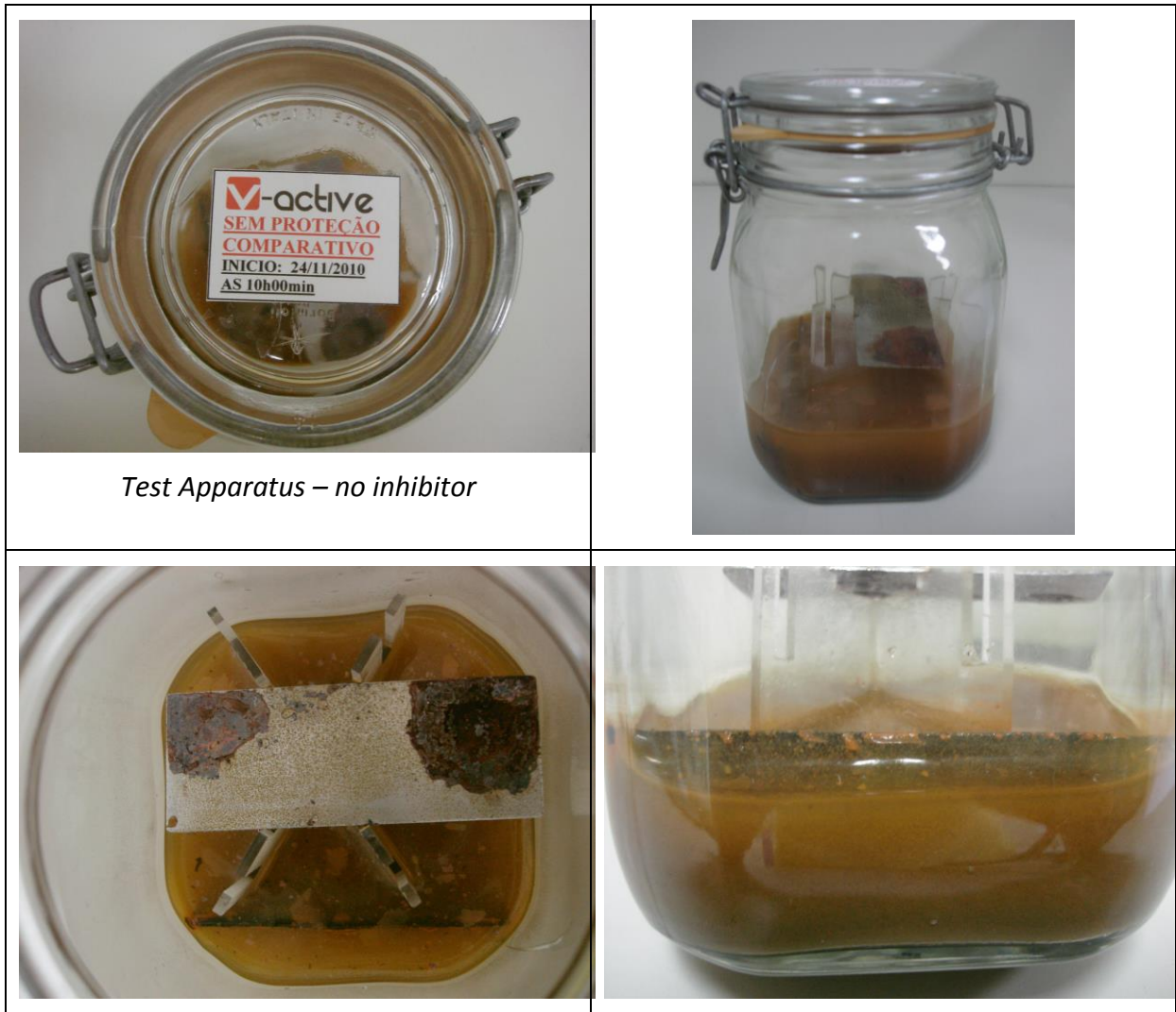
Figure 19 – Test apparatus for liquid and vapor phase – no inhibitor
