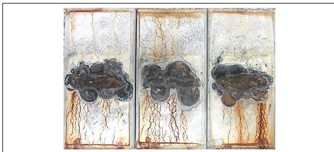
Figure 51c – Samples 04, 05 and 06 (SPH1712 wet) – after 20 cycles Cyclic Corrosion Test
