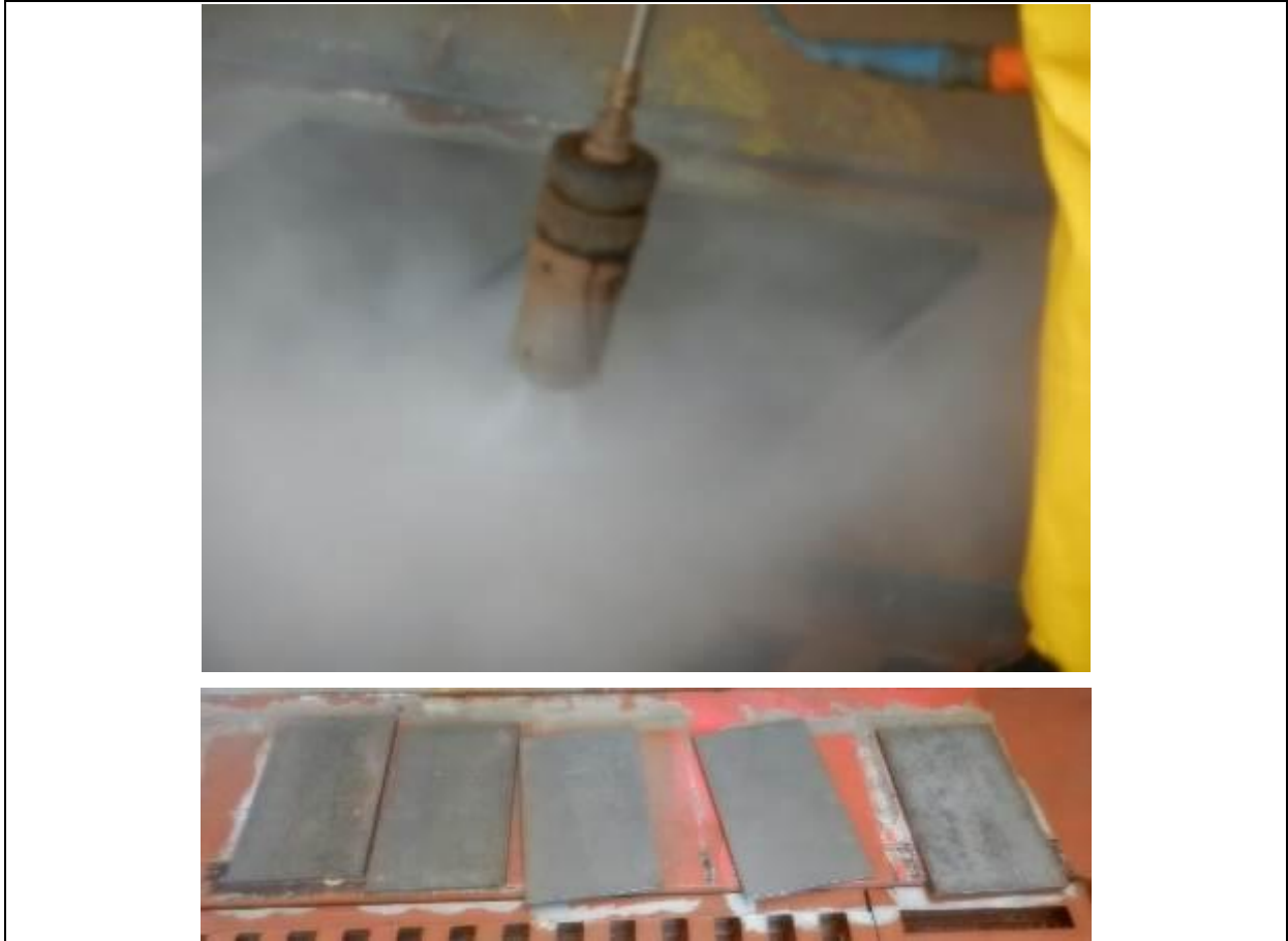
Figure 45 – Steel plates – after hydrojetting using fresh water
