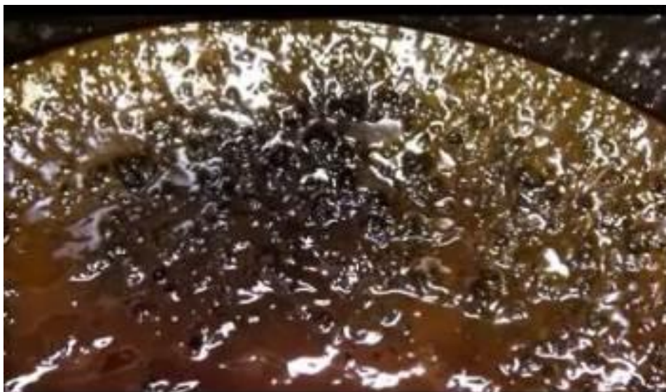
Figure 37 – 200L Drum with diesel and without corrosion inhibitor: formation of an organic mass at the bottom.
