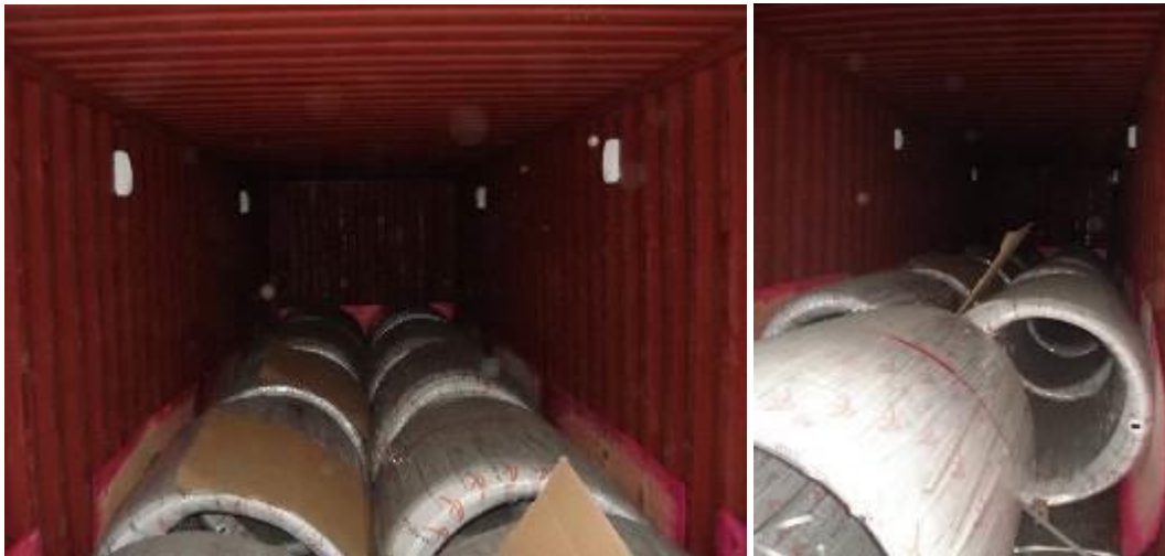
Figure 56 – Scheme of the of coils wrapped with PR VCI579 tape and FM8 after loading - 11 steel coils
