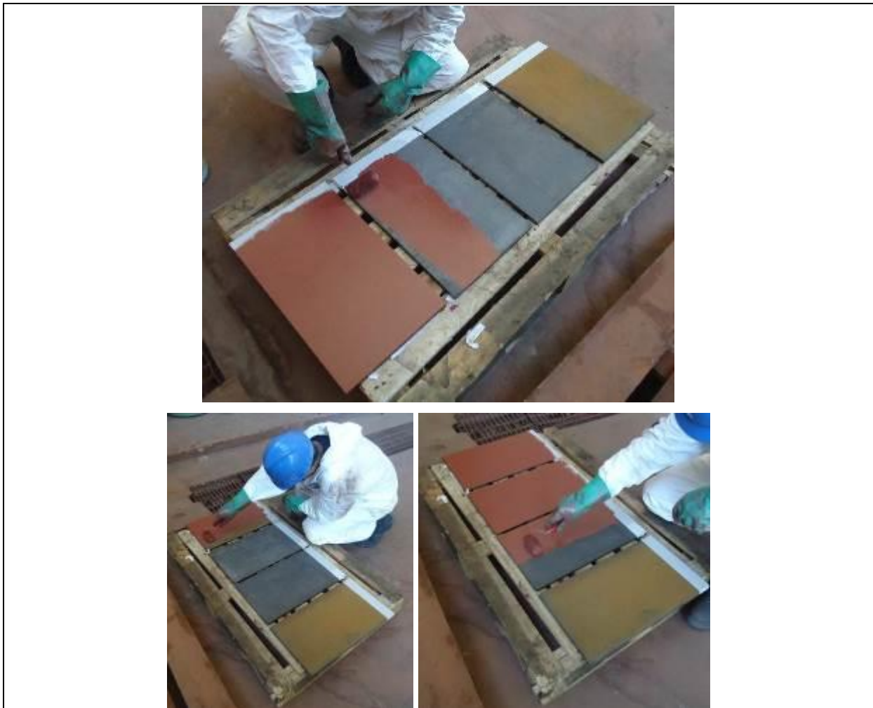
Figure 47 – Steel plates – after hydrojetting – painting process
