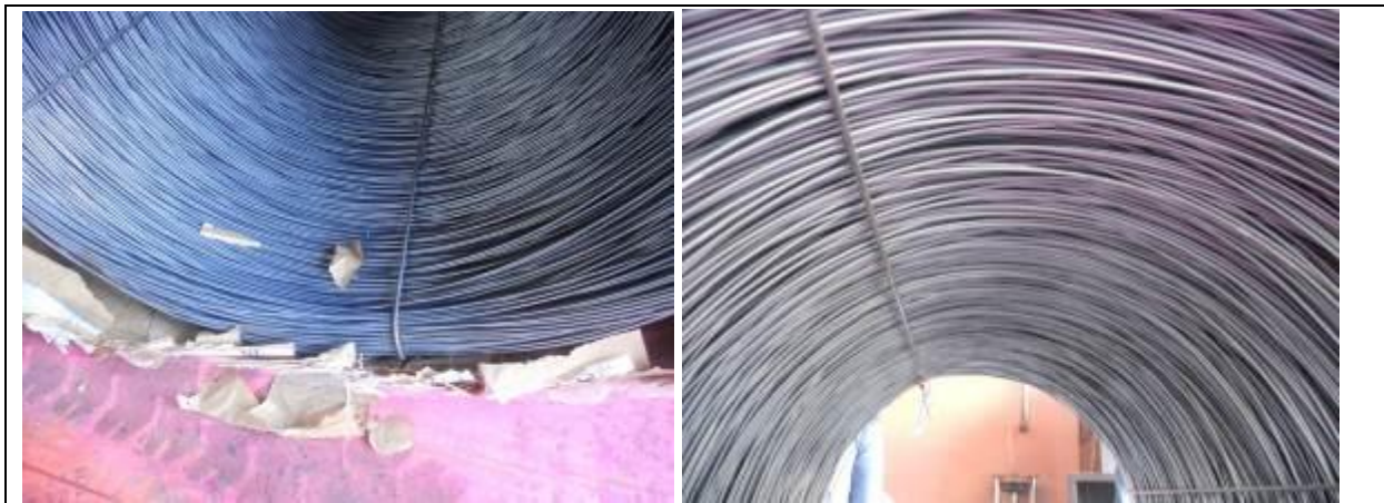
Figure 68 – Wire Steel Coil after 43 days - No oxide inside the coil.
