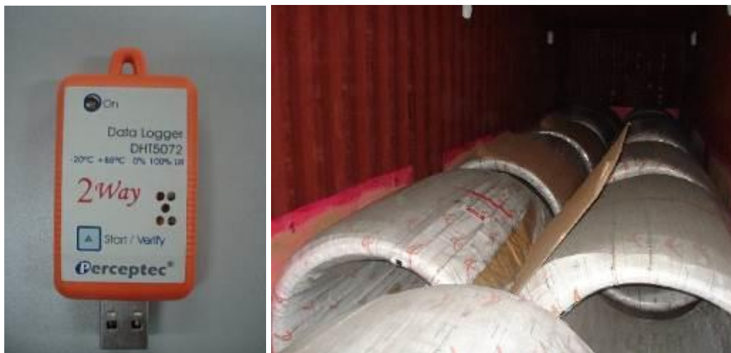
Figure 58 – Internal datalogger – inside steel coil
