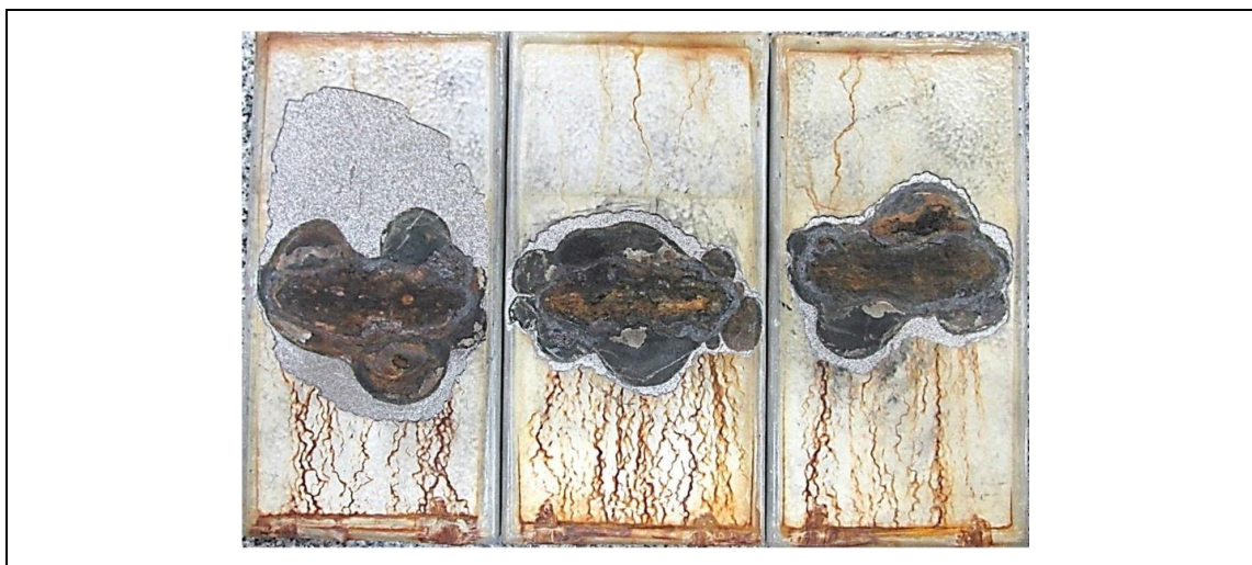
Figure 51b – Samples 01, 02 and 03 – Condition H 2 O – after 20 cycles Cyclic Corrosion Test
