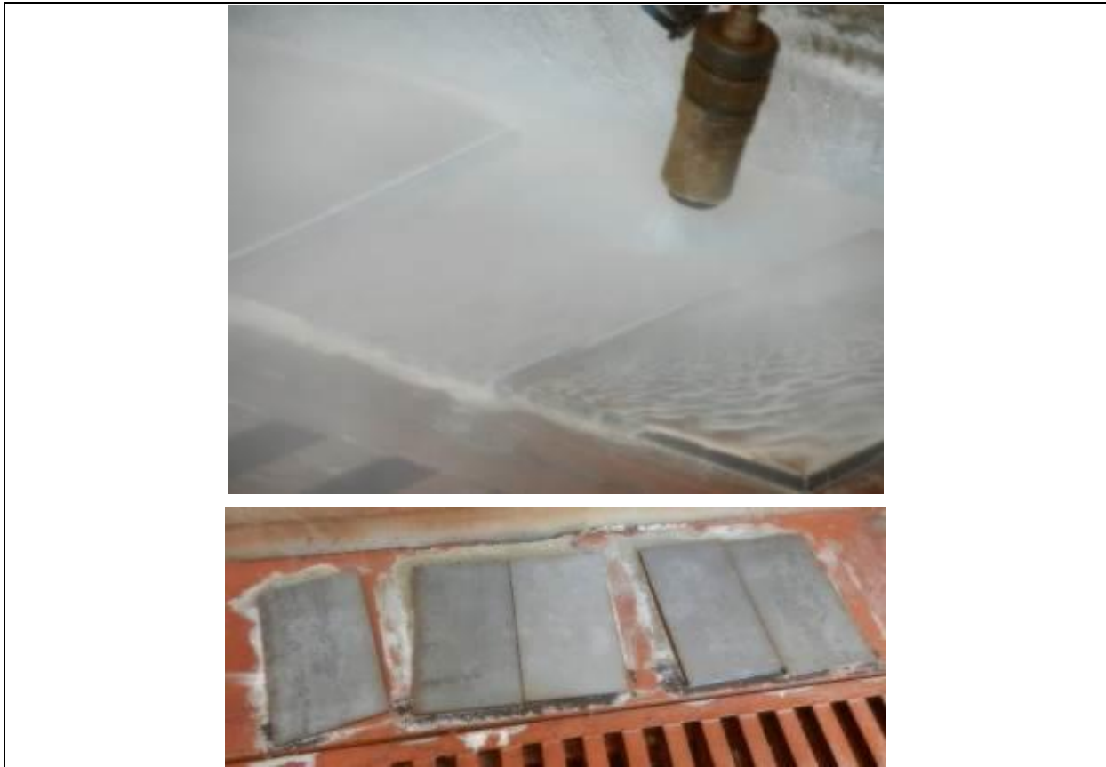
Figure 44 – Steel plates – after hydrojetting using 2% V-active VCI 1712 SPH
