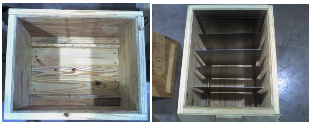
Figure 23 – Fitting metal plates (for contact and vapor analysis)
