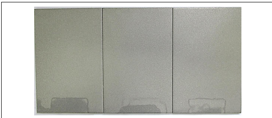
Figure 49c – Condition SPH1712 dry – 1, 2 and 3 – flash rust test – initial (time 0)
