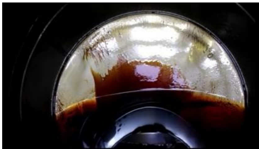
Figure 40 – Bottom of the Drum with diesel and with 0.5% of V-active VCI1061 corrosion inhibitor
