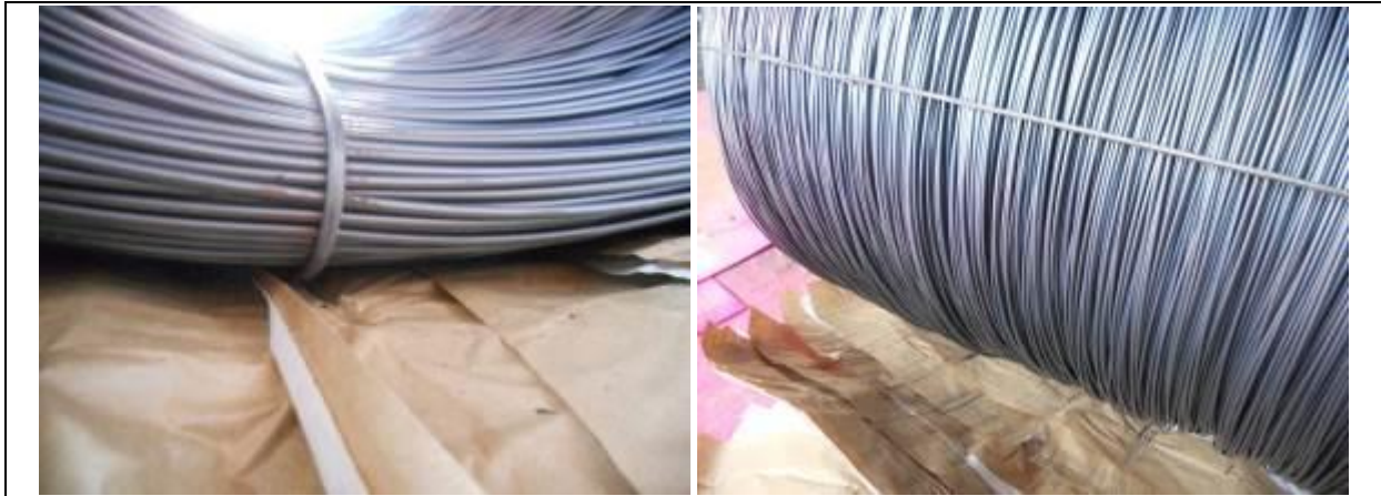
Figure 69 – Wire Steel Coil after 43 days – bottom condition
