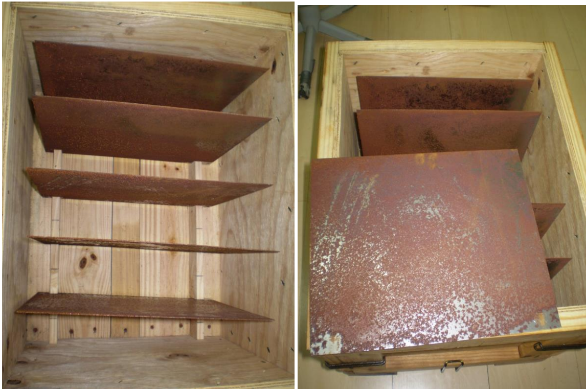
Figure 24 – Results for metal plates (no V-Active VCI)
