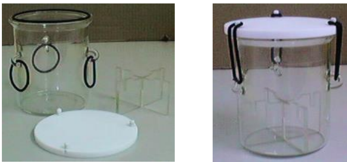
Figure 16 – Standard ABNT NBR 15109 – original apparatus
