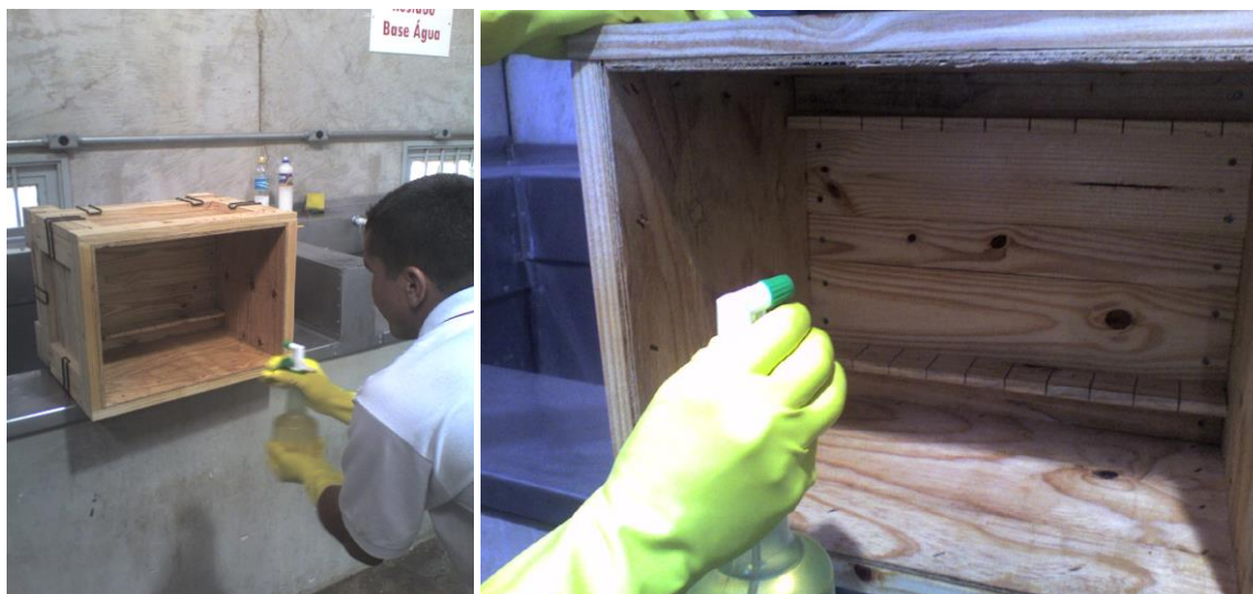
Figure 22 – V-Active VCI Treatment – by spray
