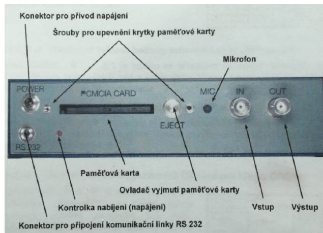
Obr. 3.3 – Horní panel defektoskopu [11]
