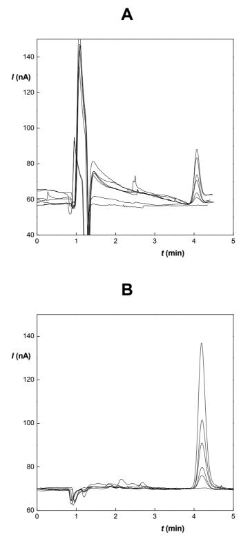
**Fig. 3**: Chromatograms of chlortoluron samples of various concentrations in matrices of river water (A) and soil (B). Column LiChroCART<sup>®</sup> 125-4 Purospher<sup>®</sup> RP-18 (5 µm), mobile phase B-R buffer of pH 4.0 and methanol (40:60, v/v), flow rate 1.0 mL min<sup>-1</sup>,  $E_{DET} = +1.3$  V, chlortoluron concentration (A) 10; 8; 6; 4; 2; 1; 0 µmol L<sup>-1</sup>, (B) 10; 7; 4; 2; 1; 0 mg g<sup>-1</sup>.
