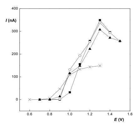
**Fig. 2**: *Hydrodynamic voltammograms of chlortoluron at CPE in mobile phase with different pH (pH 3.0* ( $\blacksquare$ ); *pH 4.0* ( $\bigcirc$ ); *pH 5.0* ( $\blacktriangle$ ); *pH 7.0* ( $\times$ )). Column LiChroCART<sup>®</sup> 125-4 Purospher<sup>®</sup> RP-18 (5 µm), mobile phase B-R buffer of selected pH and methanol (40:60, v/v), flow rate 1.0 mL min<sup>-1</sup>, injected 20 µL of 100 µmol L<sup>-1</sup> chlortoluron solution.
