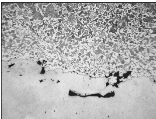
Obr. 12 Oxidy v mikro dutinách lité oceli (zv. 100x) Fig. 12 Oxides in the microvoids of the cast steel (Magn. 100x)
